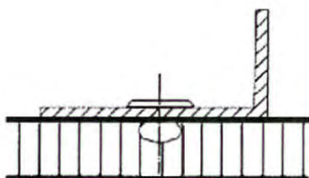
Blind rivet with panhead For ALUCORE ® with a thickness of 10mm or more
